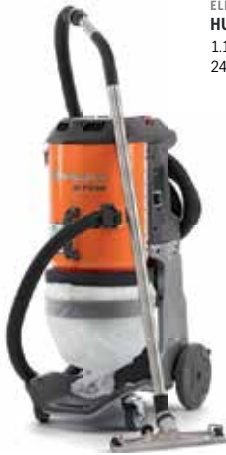
ELECTRIC-POWERED HUSQVARNA DE 110 SH 0.9kW, 220–240V, 4A, 215m 3 /h, 25kg.
